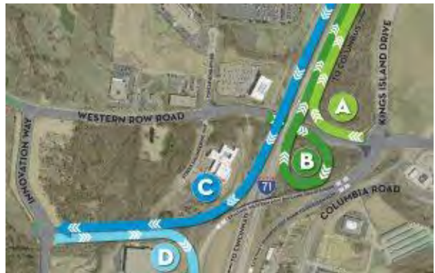
Major initiatives include working with the Warren County Transportation Improvement District on a nearly $21 million project to convert the existing Interstate 71 and Western Row Road (I-71/WRR) interchange into a full interchange with new ramps and auxiliary lanes completed February 2019. Additions include (A & B) Access to Northbound I-71, (C) Southbound off I-71 to Innovation Way, and (D) 2 nd Access to Southbound I-71.
