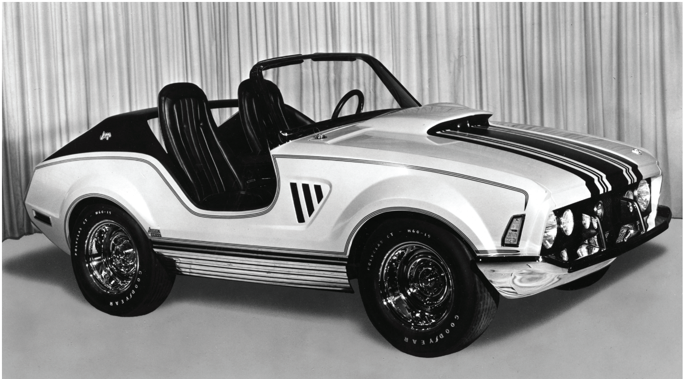
The XJ001, a Jeep Corporation concept car from approximately 1965, was created for the New York International Automobile Show. The idea car was 4-wheel drive, four speed transmission, a modified CJ-5 chassis, and a full fiber glass body. Photo courtesy of the Lucas County Libraries Archives.
